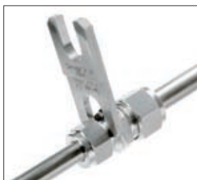
Properly tightened, the gauge will not fit
