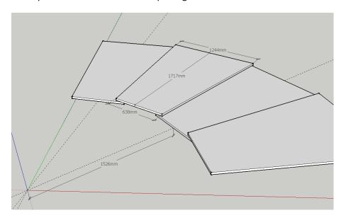
Trapezoid; Delta R = 1717mm, Long Base 1244mm, Short base 638mm. Overlap is 50mm on each side for structure and internal service passage. Inner radius is 1526mm.
