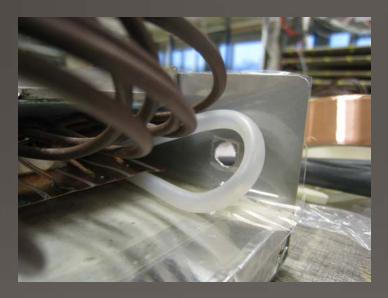
• Signal cable twist and pressure
