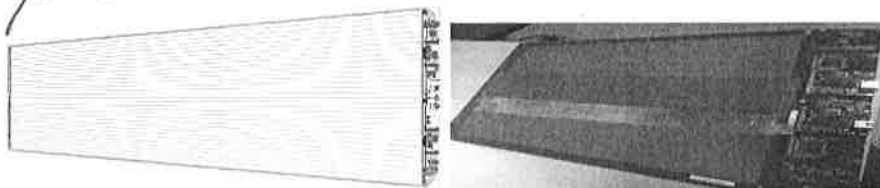
Figure 5.27: Left: Schematics of a large Active Sensor Unit (ASU) with pickup strips read out from both ends by two independent channels of the the same PETIROC. ASICs and TDC on FPGA mezzanines are placed on the outer radius. Right: a picture of a realized small size ASU following the same schematics with pickup strips in the middle.
