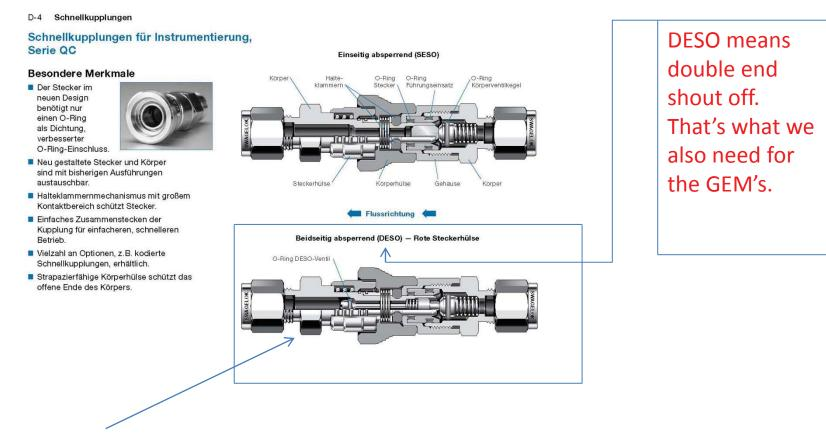
This kind of connectors are used for the CMS drift tube muon chambers. But for Gas. So it was possible to use brass. We need stainless steel.
