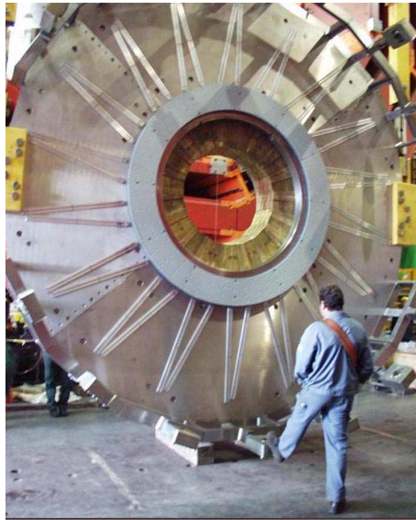
Figure 7.3: CMS HE back-flange showing GE1/1 chamber support rails.
