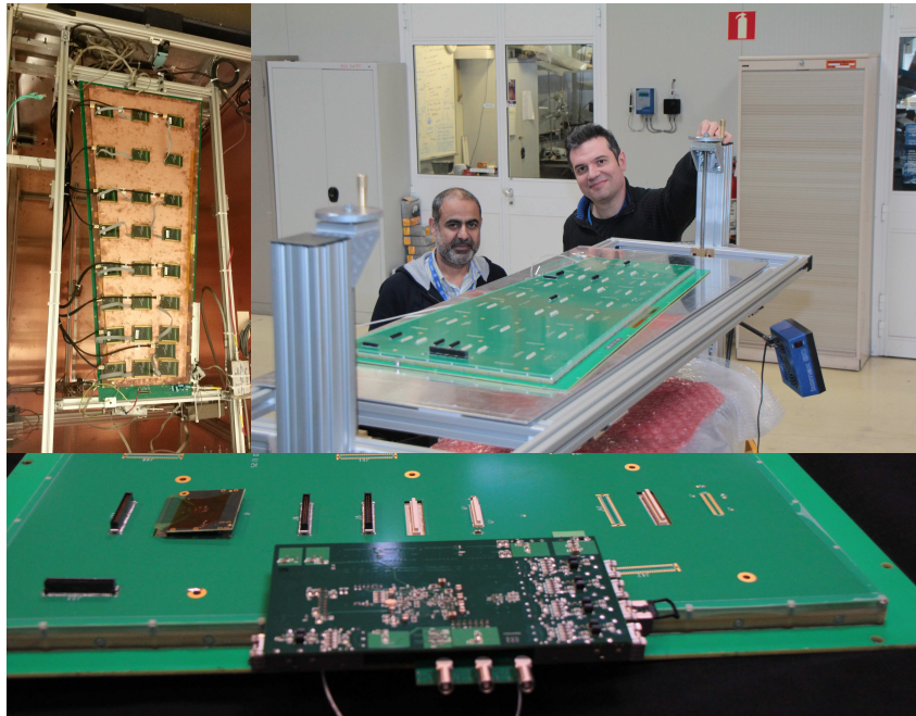
Figure 1.6: Most recent GE1/1 chamber prototypes (top left) in the uniformity test stand, (top right) ready for CSC-GEM integration tests and (bottom) latest version of Optohybrid mounted on detector.
