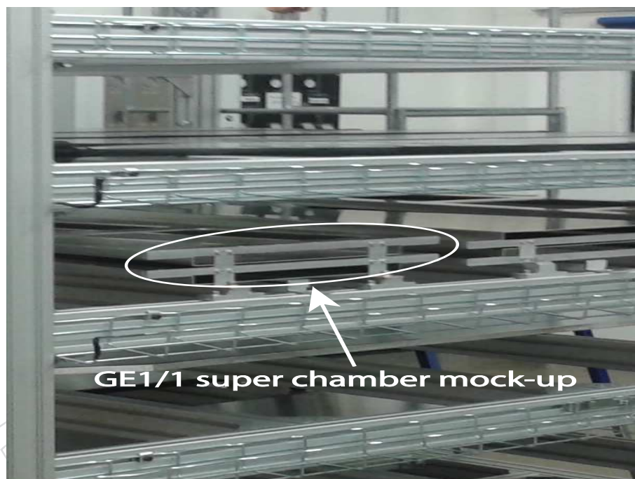
Figure 5.12: Schematic view of the Cosmic Stand at CERN. In the picture are visible the two mock-up of a GE1/1 superchamber. The cosmic stand can accommodate up to 15 superchambers
