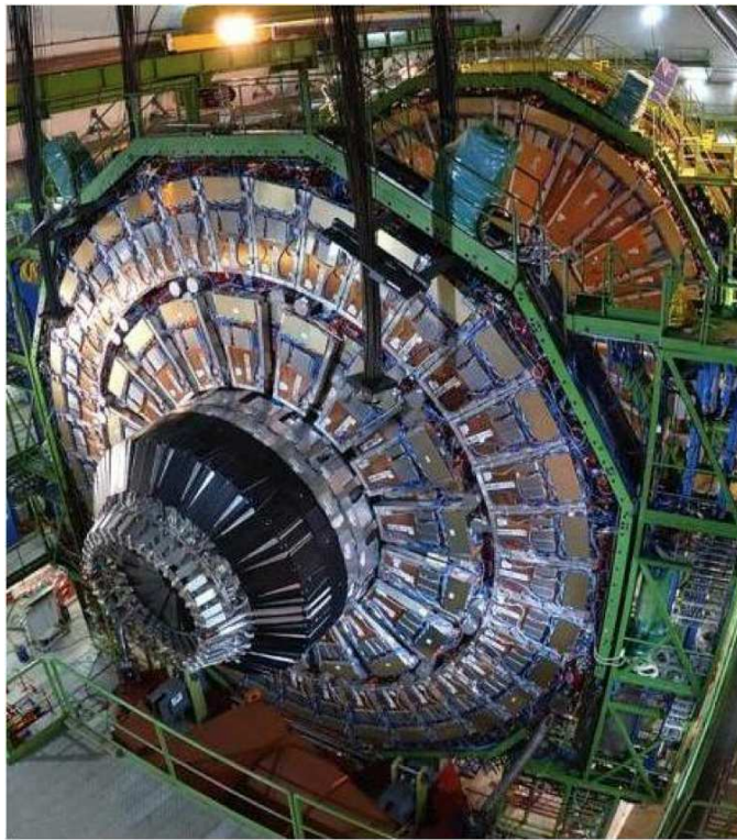
Figure 2: The CMS Endcap YE1 disk showing the “nose”, namely the high- \eta region.
