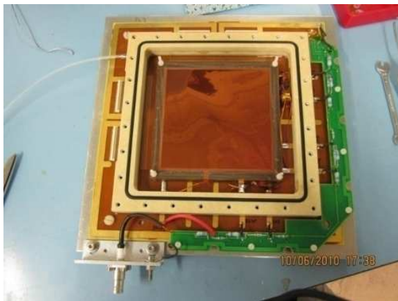
Figure 9: The standard double-mask Triple-GEM prototype. Left: Detector during assembly. Right: Configuration of gaps between electrodes.
