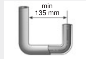
● Minimum clearance of U-shape bends
