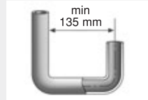
● Minimum clearance of U-shape bends
