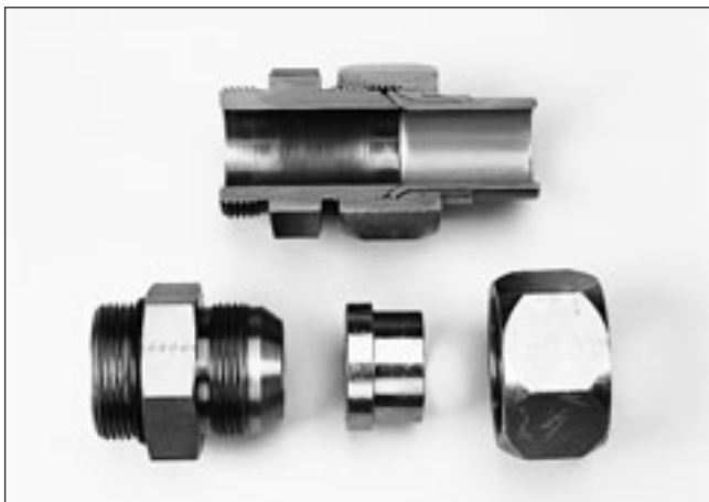
Fig. C1 – Triple-Lok® fitting components (fitting body with O-ring, sleeve and nut) and assembled Triple-Lok® fitting cutaway
