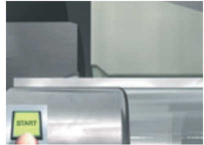
After starting the process, the dies clamp the tube and the forming pin starts to move forward
