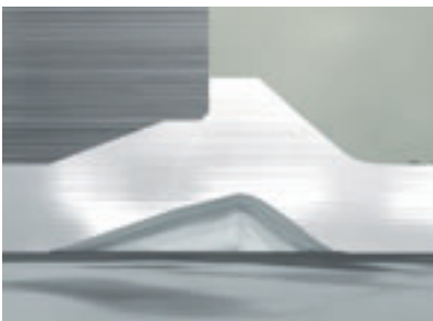
As soon as the moving pin touches the clamping jaws, the forming process is completed
