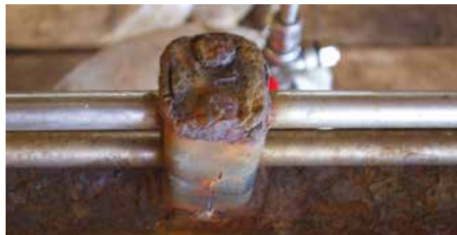
Crevice corrosion between the tube/tube trap interface.
