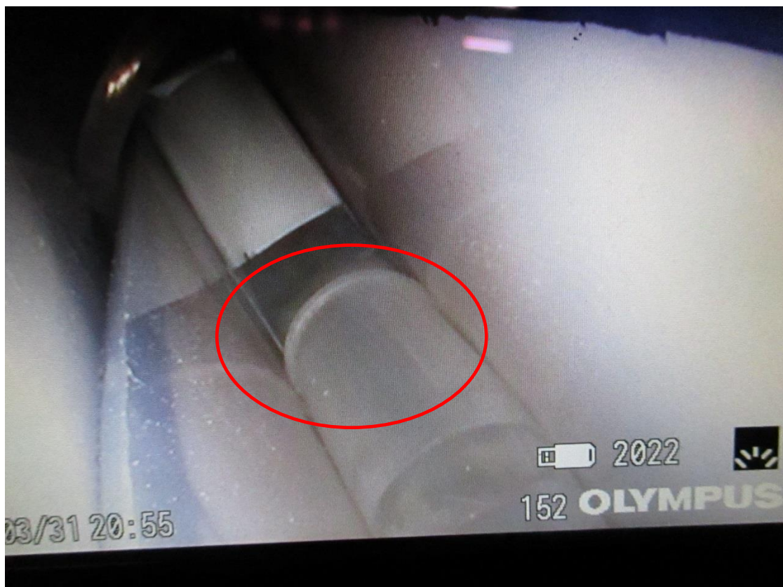
Increase in end diameter due to excessive heating
