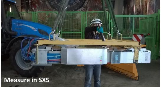
11AM Rad levels are comparable to background contamination in UXC55. Chamber can be moved to ME1/1 lab area and disassembled
