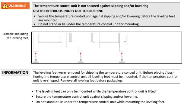
• Do not lower the temperature control unit until all leveling feet have been mounted.
