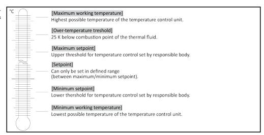
The workings of the overtemperature and low-level protection depend the type of temperature control unit.
