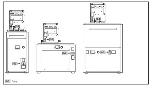
The thermal overcurrent circuit breakers for all-pole disconnection (L and N) are located at the back. In case of a fault (no function and/or no display) please first check if the overcurrent circuit breakers have tripped. If the overcurrent circuit breakers trigger again immediately after reversing, please unplug the power cord and contact Customer Support immediately. → Page 92, section »Contact data«.
