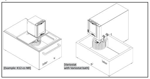
Note the volume displacement caused by a sample (e.g. Erlenmeyer flask). Place your sample into the empty bath. Only then fill in a sufficient amount of temperature control medium. Also note that the level of the temperature control medium drops when you remove the sample. This may cause a safety shutdown (low level protection) during an enabled thermoregulation. Therefore, switch off the temperature control unit beforehand.
