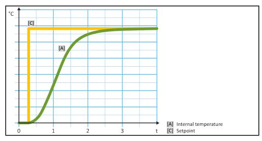
Internal, dynamic temperature control with possible overshooting of the temperature
