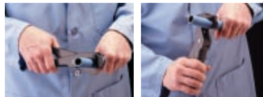
The rotating/rocking technique produces fast easy cuts.
