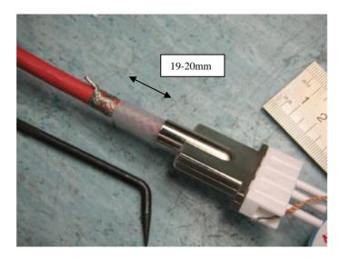
Position the smaller TRT over the ground wire and up against the housing entry. Do not put in onto the outside of the housing. Heat to full retraction using thehot air gun set to #5 on the Model ......
