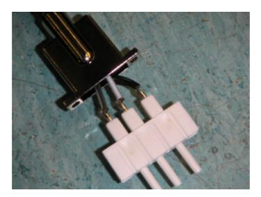
Gently slid the housing down the cable so tomate the housing and base .
