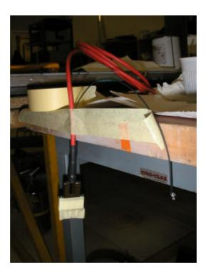
Tape up the interface between the base and housing to ensure no leaks of epoxy. The epoxy must continue to drip easily ( and annoyingly ) from the needle. Inject through the 2 holes in the top of the housing , inserting the needle fully but carefully so as not to damage the insulation of the cables. The pressure required is quite firm. Fill completely the housing to the brim and allow any bubbles to escape. Add a few drops more as the epoxy retracts on reticulation.
