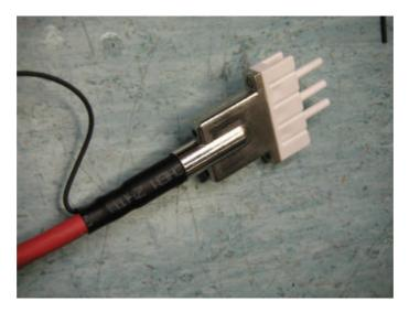
Position the large internally coated TRT over the ground wire and up against the shoulder of the connectors housing . Using the Hot air gun a s before heat the TRT starting from the connector end. Solder on the ground connection lug SCEM...... After having cut the wire to 120mm ??????
