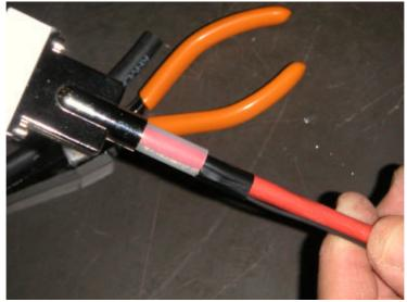
Cut the individual conductors to 27mmin length. Using the Thermo denuder [Hot Weezers] strip the individual wires overva length of 5mm at their ends. Twist the two black thinner wires together . Using soldering iron tip 'ETB' set to 400°C and 2% Ag solder.tin all three ends. Thread the white cable through the two black cables as it will connect to the centre pin.
