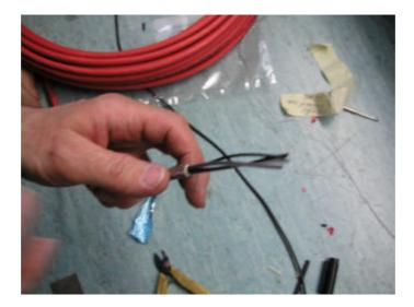
Pull out the strands of the shield braid using a scribe . Twist the ends together for soldering to the ground wire connexion.
