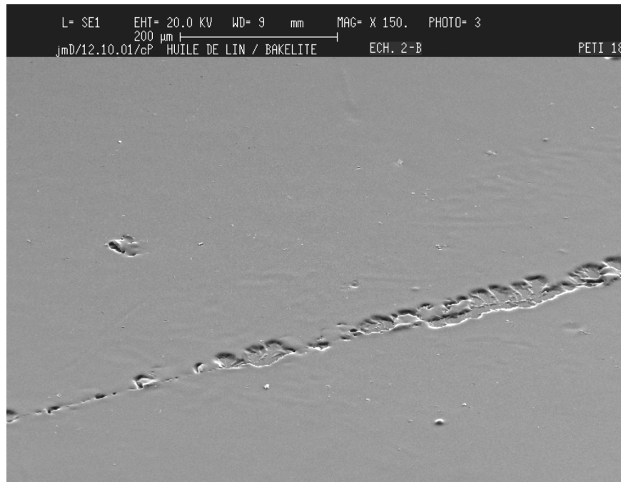
General surface observation. Tilt 60°. Some uncoated areas and inclusions.
