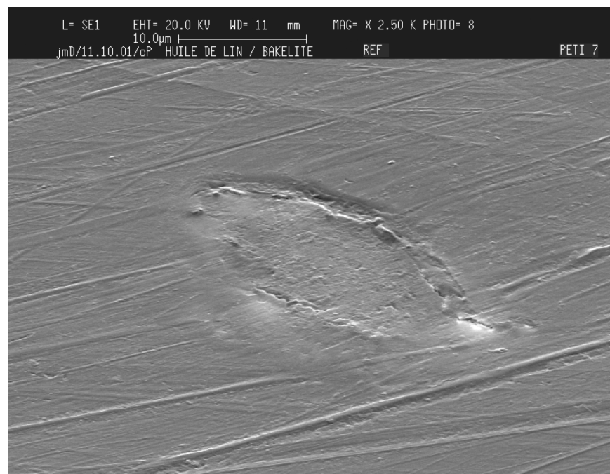
An oval surface non-uniformity : detail of flow 3 of the first photo.
