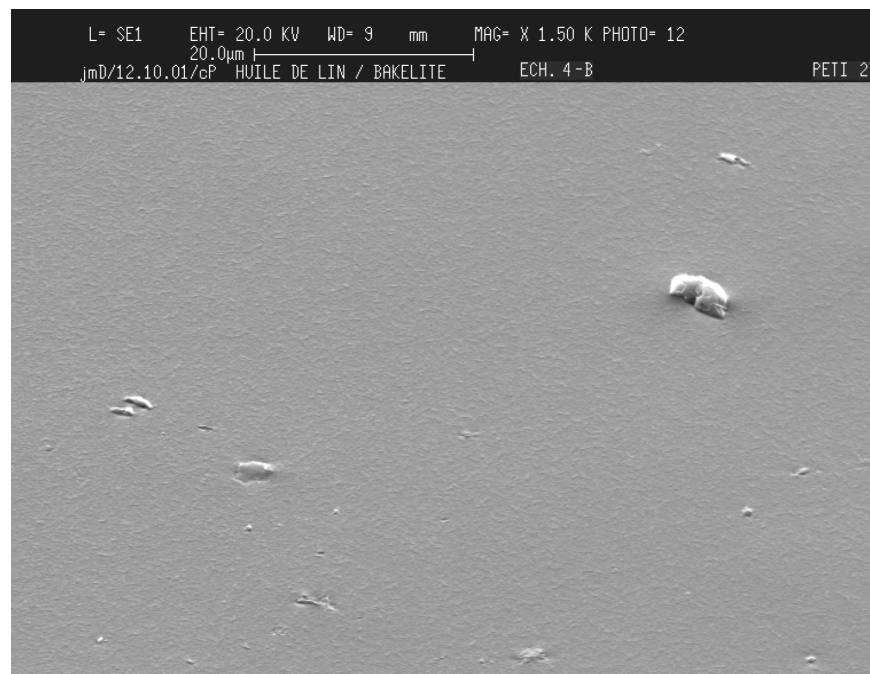
Detail of the inclusions and dust particles.
