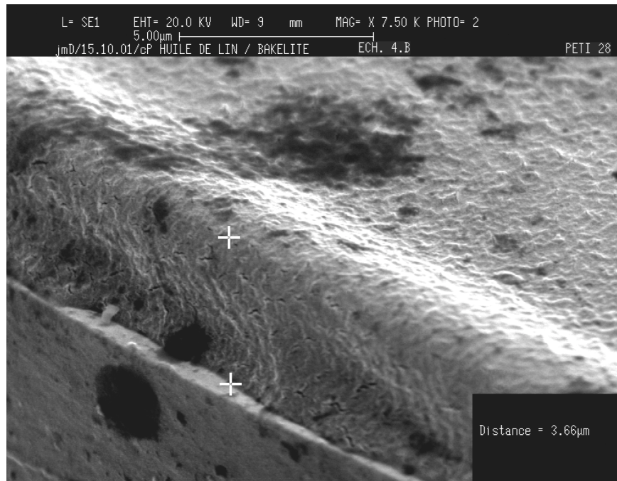
The thickness of the coating layer = 3.7 µm
