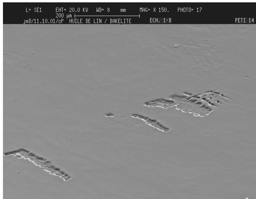
The coating layer is clean and smooth; bad wettability for certain areas.
