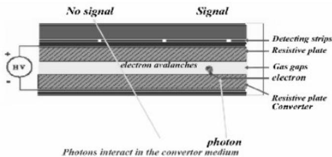
FIGURE 2. General construction of RPCs as PET detectors.
