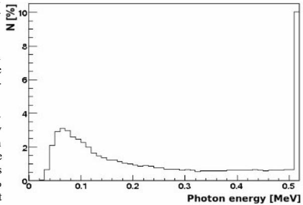
FIGURE 3. Energy spectrum of the photons, leaving the human body.
