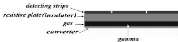
FIGURE 4. RPCPET: GC (gas – converter) design
