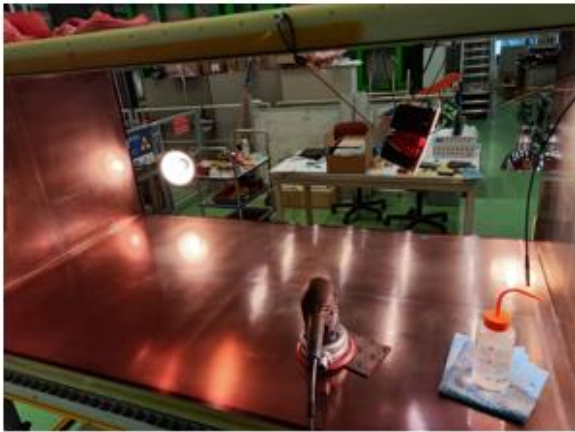
Inner cage surfaces polishing
