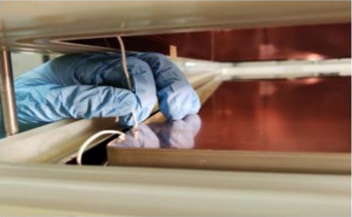
Connection of last strips to cathode and to high voltage feedthrough
