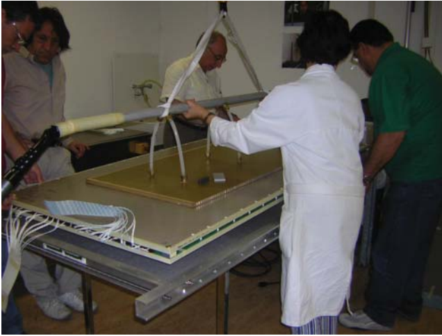
Figure A.21 The vetronite/glass stack of one of the MRPCs of the EEE experiment while it is positioned inside the relative metallic box. (From La Rocca et al. , 2017.)
