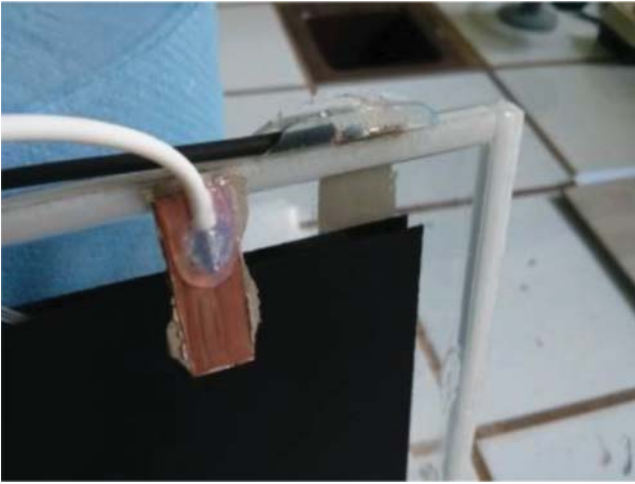
Figure A.11 High-voltage connections: The white cable is the high-voltage cable, while the black one is the ground cable, connected to the opposite side of the RPC. (From Loterman, 2014.)
