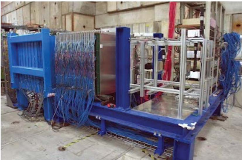
Figure 9.37 Photograph of the DHCAL setup at CERN showing the main stack with tungsten plates followed by the TCMT (tail catcher/muon tracker) with steel plates. (Adams et al. 2016. Reproduced with permission of IOP Publishing.)
