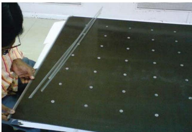
Figure A.6 Photograph of the spacers assembling process on a 1 \times 1 \text{ m}^2 Bakelite electrode. (From Biswas, 2010.)
