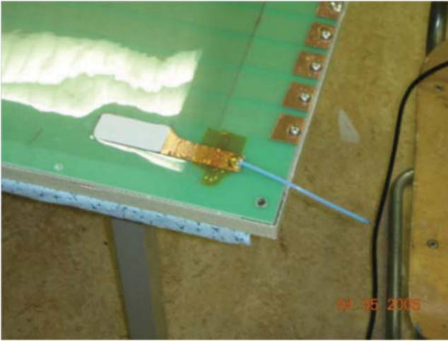
Figure A.18 High-voltage connection on an MRPC of the EEE experiment. (From La Rocca et al. , 2017.)
