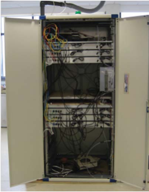
Figure 9.15 Picture of the system built at Bristol University for muon scattering tomography with RPCs. The six aluminum cassettes contain two RPCs each, providing X and Y coordinates. High and low voltage cables and data connections are visible. The gas mixers are located at the bottom. (Baesso et al. 2014. Reproduced with permission of IOP Publishing.)
