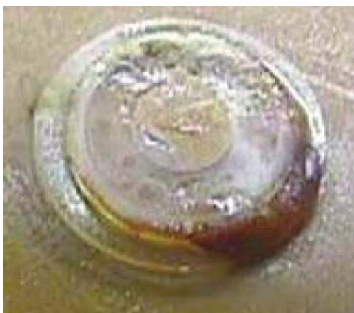
Figure 6.21 A spacer taken from one of the BaBar RPC chambers; the accumulation of brown linseed oil on the bottom right (a dark spot in a black and white version of the photograph) of the spacer can be clearly seen; for the colour version see (Va'vra, 2012).
