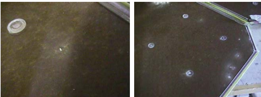
Figure 6.24 Whiskers formed onto the cathode of two BaBar RPC chambers. (From Va'vra 2012.)
