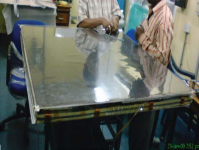
Figure A.8 Photograph of a fully assembled RPC, wrapped in a shielding foil. (From Biswas, 2010.)
