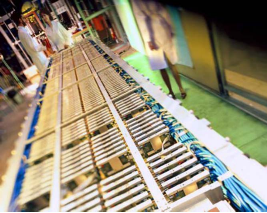
Figure 5.42 One of the ALICE TOF MRPC supermodules. (ALICE Collaboration 2008b. Reprinted with the permission of CERN.)
