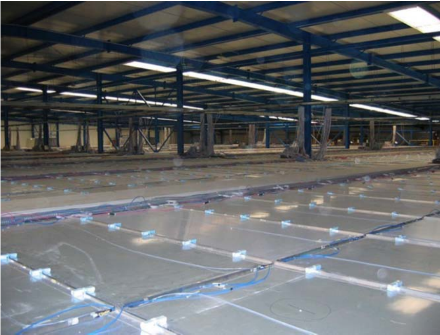
Figure 5.20 Picture of the experimental hall hosting the ARGO-YBJ detector. The carpet of RPCs is well in evidence. (Surdo and on behalf of the ARGO-YBJ Collaboration 2008. Reproduced with permission of Elsevier.)
