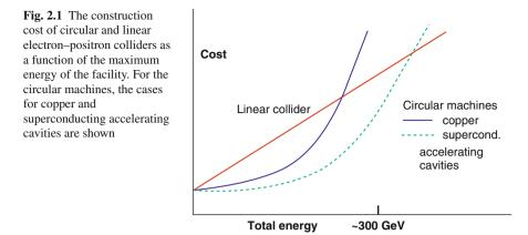
a machine with only 3 times the energy of LEP the radius of a circular machine becomes unrealistic (several hundred kilometres in circumference). Since the design energy of LEP was well below the crossover of about 300 GeV, only a circular machine had to be considered, no matter what kind of accelerating cavity was considered.
