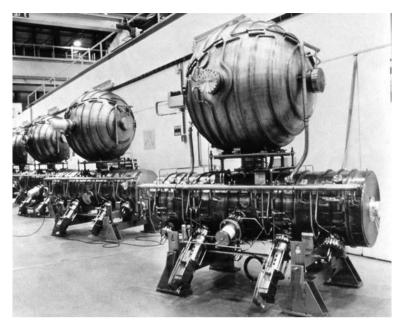
Fig. 6.8 Several copper units of the accelerating and storage cavity
