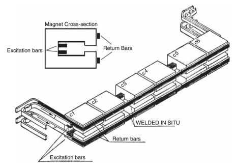
Fig. 6.5 The electrical excitation of the bending magnets
