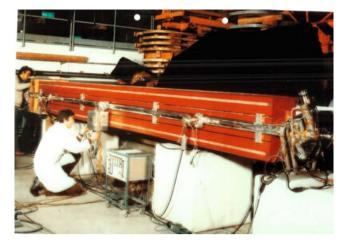
Fig. 6.3 A 'concrete' magnet during testing
