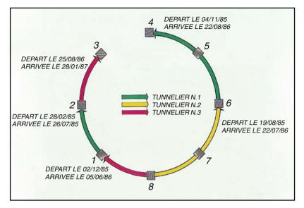
Fig. 4.8 The tunnelling split up into different sections for three machines with rotating heads; the remaining part was excavated using explosives
