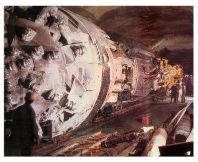
Fig. 4.7 Rotating head of the tunnelling machines. The front head carries rolls which break the rock
