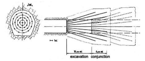
Fig. 4.13 The arrangement of stepped pilot borings
