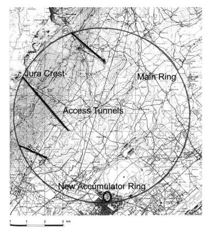
**Fig. 2.2** The LEP position in the first proposal ('Pink Book'). The ring passes deep under the Jura crest; three long access galleries were necessary to provide access to the underground halls at points *P3*, *P4* and *P5*. A new accumulator ring under the old Intersecting Storage Rings (ISR) tunnel was also proposed
