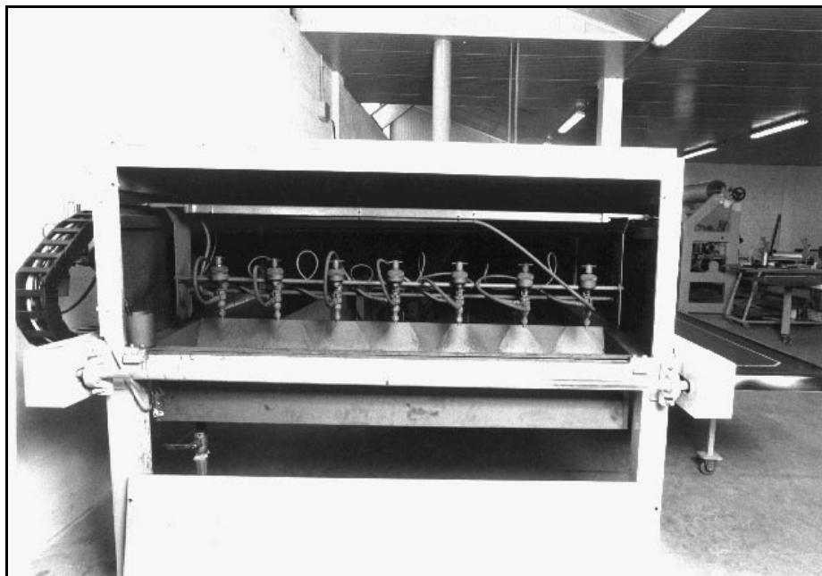
Fig. 5.3.2: The RPC graphite spraying facility.
