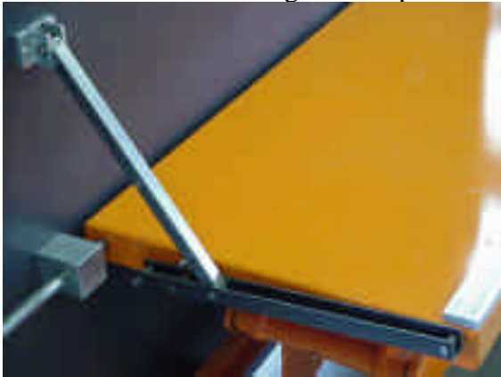
Mechanism for blocking vertical position
