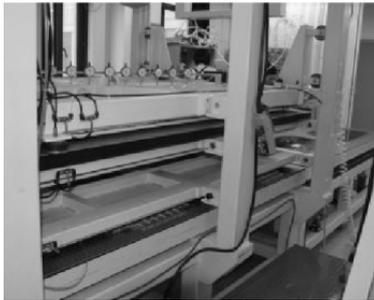
Figure 3. Facility for the assembly of gas gaps. The facility equipped with 3 sets of flat metric tables and rubber chambers enables three consecutive assembly procedures.
