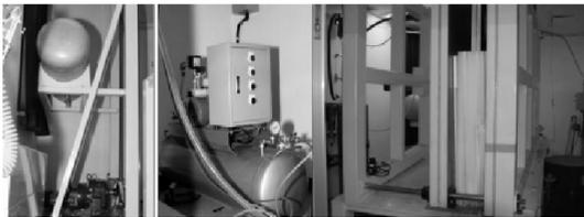
Figure 4. Oil coating facility. The 200 l oil tank and the lifting device are shown in the left figure. Before oiling, the gas gaps are vertically mounted inside a pressing device, as shown in the right picture.
