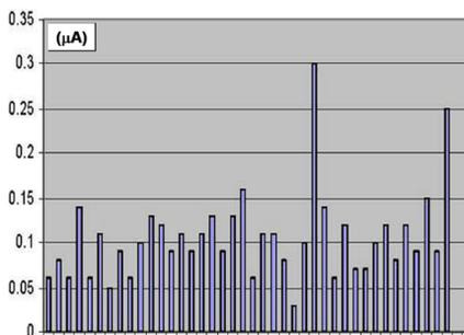
Figure 7. Result of the HV test on 40 good gas gaps (the unit of vertical axis is  $\mu\text{A}$ ).
