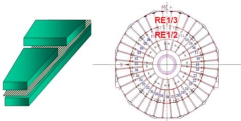
Figure 3. Three gas gaps in a low  $\eta$  RE chamber (left) and the view of the first station in RE system (right).
