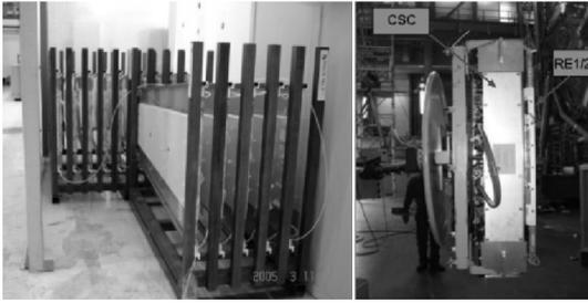
Figure 8. Completed RPCs (left) and the mated CSC+RPC (right).
