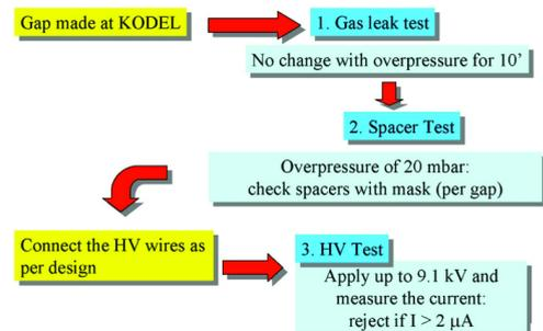
Figure 6. Gap QC in Korea, which is repeated at CERN.
