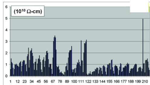
Figure 5. Volume resistivity (unit of  $10^{10} \Omega\text{-cm}$ ) measurement on 220 bakelite sheets.
