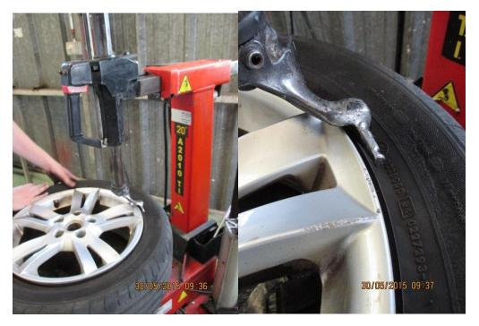
The head will move away from the wheel rim automatically to ensure the wheel is not damaged later in the process.
