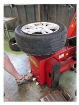
Before bringing the arm down release the red trigger.
