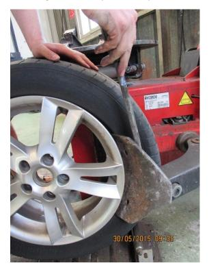
Rotate the wheel 30- 50dgrees at a time and work the tyre from the rim. Older tyres/rims can be VERY stubborn !
