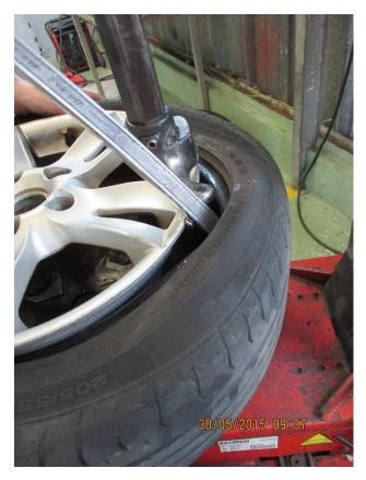
It is levered back to bring the tyre bead over the duck's head.
