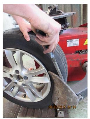
The wedge end of the press must penetrate between the wheel and the tyre. This is not always easy.
