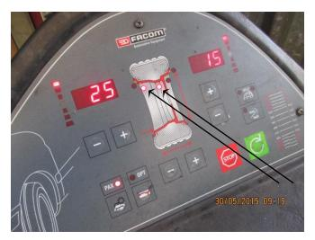
Rotate the wheel by hand to find the two different positions around the wheel periphery .
