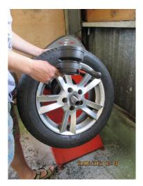
Use the specific clamp plate for alloy wheels to avoid damage.
