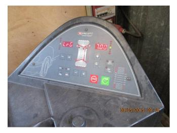
Here a wheel width of 7 inches is shown. This value was put in using the button shown
