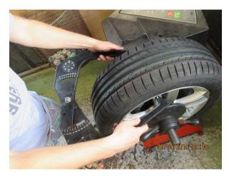
The wheel diameter can also be measured using this device or simply read off the tyre.
