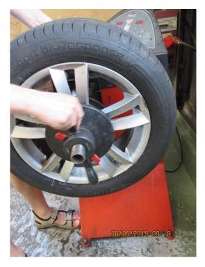
Take the three parameters of the wheel/tyre assembly, namely inner diameter off set (mm), wheel width (inches) and wheel diameter (inches).
