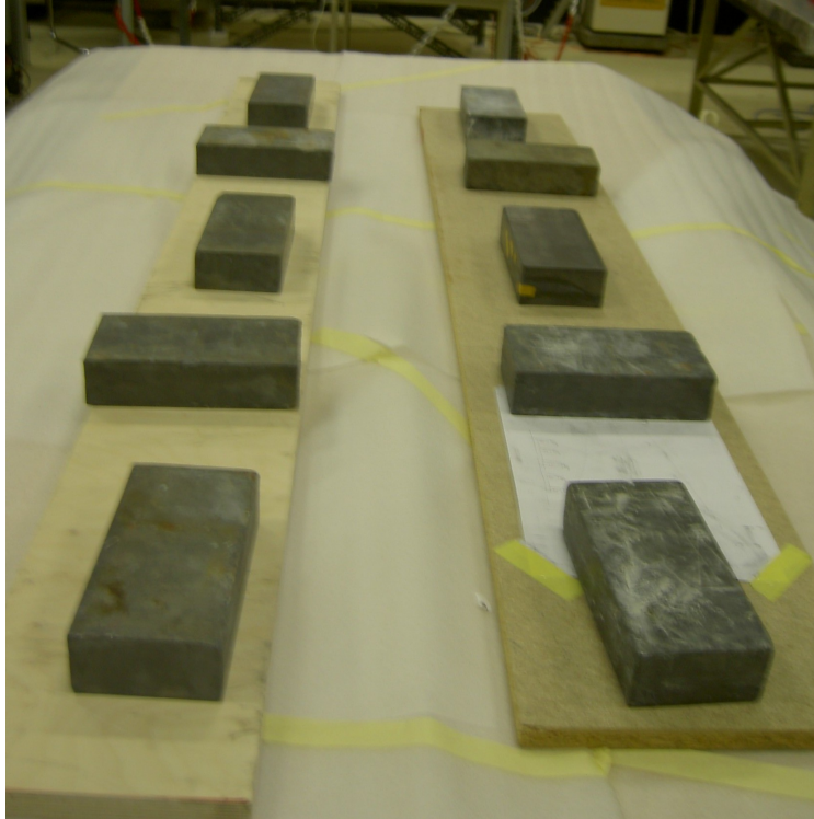
Figure 6: Distribution of lead bricks on top of bent gaps.
