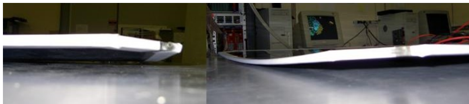
Figure 3: Bent RE1/2 gas gaps. Notice that in the image on the left, one can see right underneath the gap as a consequence of the lengthwise curvature.
