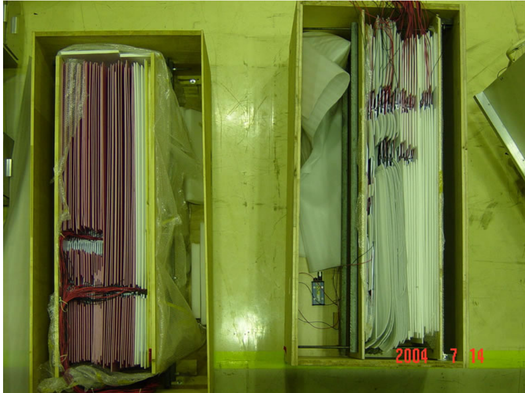
Figure 2: Storage of gas gaps for shipping. The metal clamp used to keep the gaps vertical can be seen in the crate on the right.
