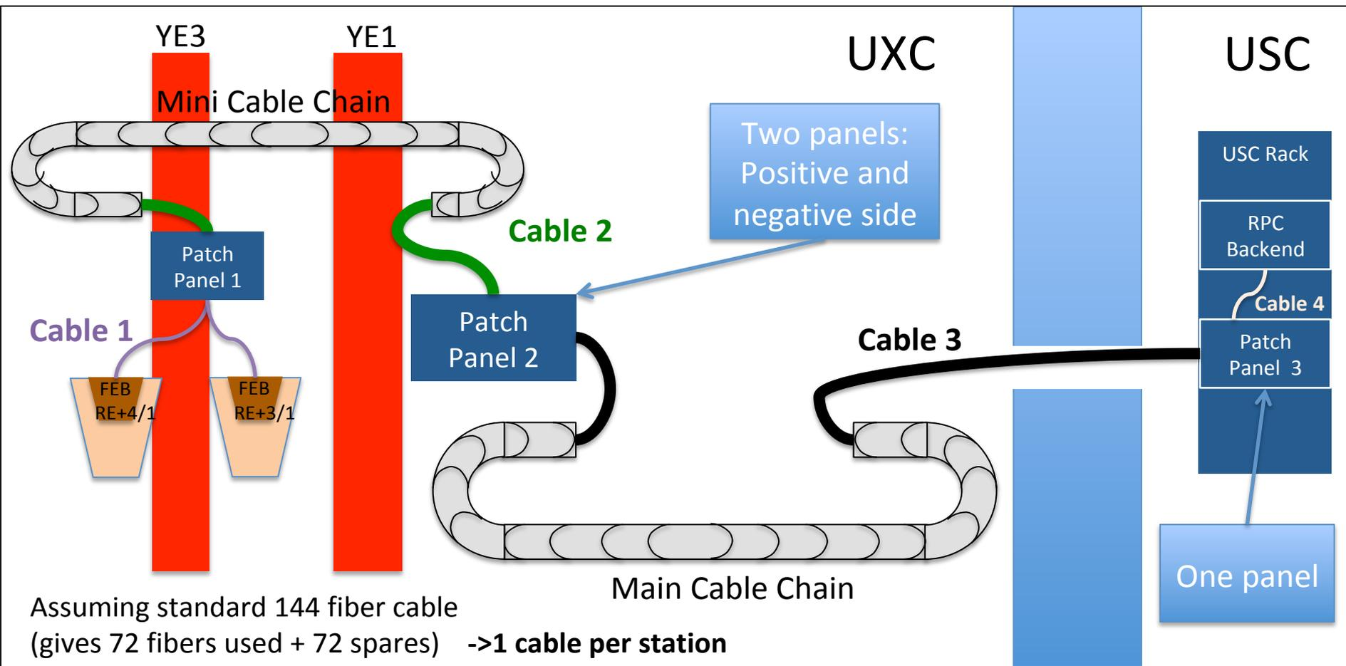
To be installed 72 Chambers in total.
