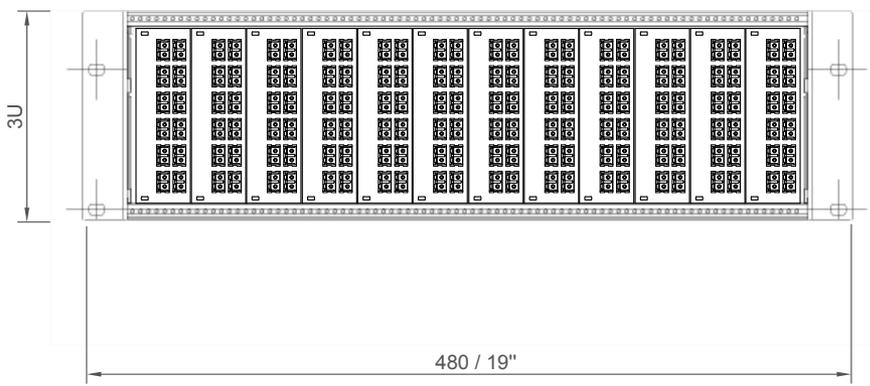
Proposed material for the "patch panel 2" is plastic PC/ABS.
