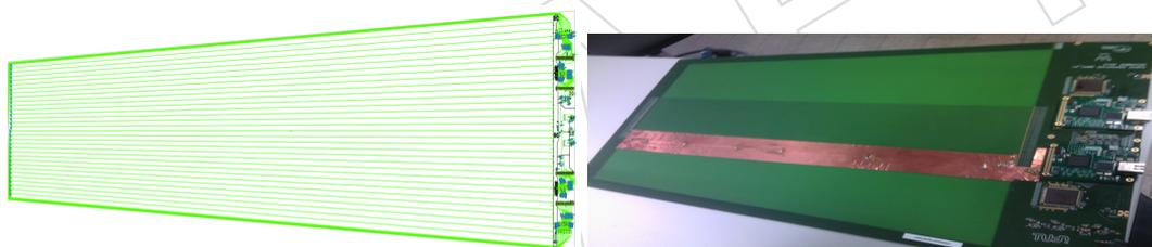
Figure 29: Left: Schematics of a large ASU with pickup strips read out from both ends by two independent channels of the the same PETIROC. ASICs and TDC on FPGA mezzanines are placed on the outer radius. Right: a picture of a realized medium size ASU following the same schematics with pickup strips in the middle.
