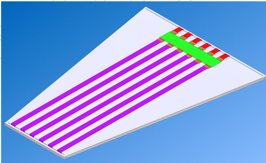
Figure 14: Scheme of the new electronic readout. The mezzanine is in green and the coaxial cables coming from the two ends of the strips ( violet and red flat cables) are connected to the mezzanine through matching small orange cards. The detector and the strips-PCB are inside the cassette and not visible here
