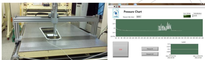
Figure 24: Test facility for the mechanical qualification composed of a metric table and a gantry arm equipped with a pencil-shape probe (left) and a pressure chart of testing the spacer failure and the gas tightness (right).
