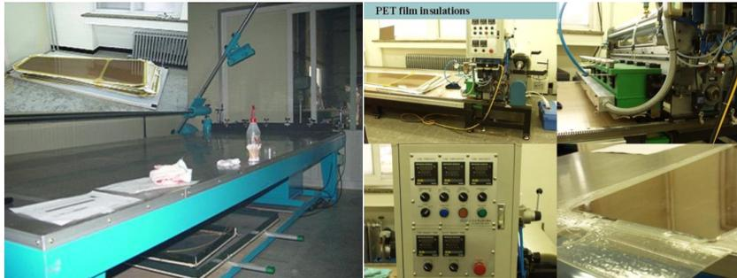
Figure 22: Operation table and the accessories of the graphite coating (left) and an extrusion facility and the control device of the PET film coating (right).
