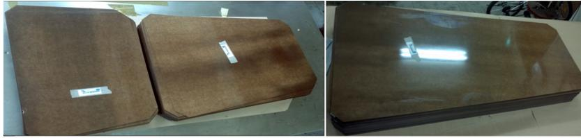
Figure 21: A batch of qualified HPL electrodes produced for the previous RE1, RE2, and RE3 RPCs.
