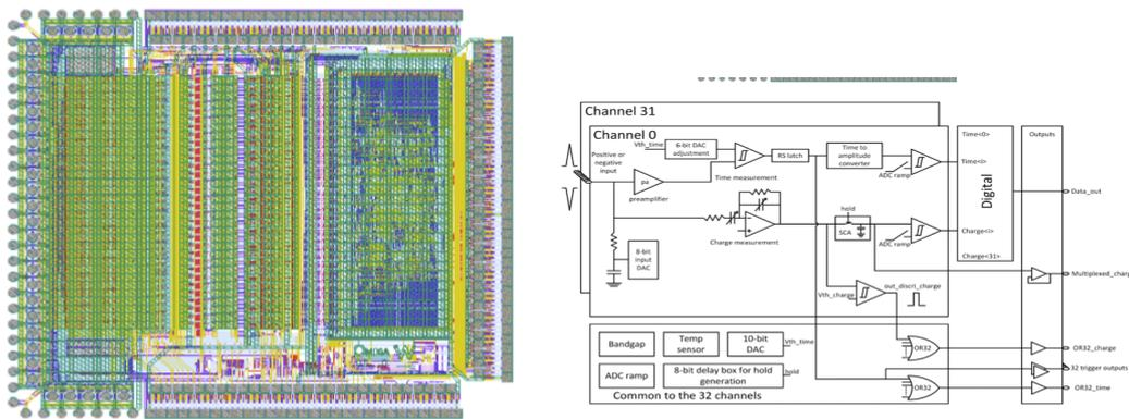
Figure 26: The PETIROC ASIC (left) and its schematics (right).
