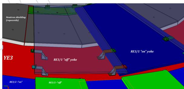
Figure 34: Schematic view of the mounting of RE3/1 chambers on the YE3 steel plate.
