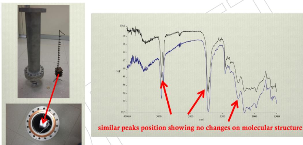
Figure 8: Left: Reactor used to test the RPC materials exposed to HFO-1234ze component. Right: FTIR spectra comparing exposed and not exposed samples after a period of 4 months. No evidence of difference in the molecular structure
