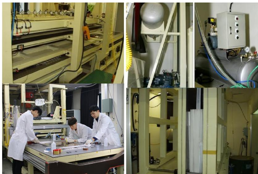
Figure 23: Flat metric tables, rubber chambers for pressurization, specially machined jigs to fix the spacers and the peripheries to assemble the gas gaps (left) and oil coating facility composed of two oil tanks, one lifting device, two air pumps, one air compressor, and a press device (right).
