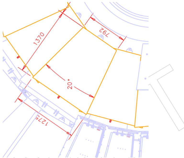
Figure 11: Detector envelope for the RE4/1 chambers.
