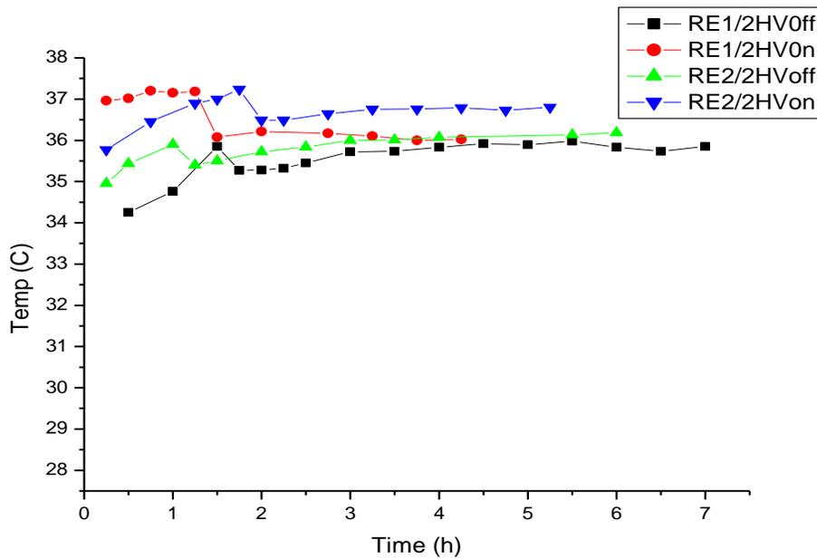
Figure 4. The variation of the FEB temperature with time for both RE1/2 and RE2/2 with HV on and off and cooling (20 °C) off at the first part of the graph and on at the second part.
