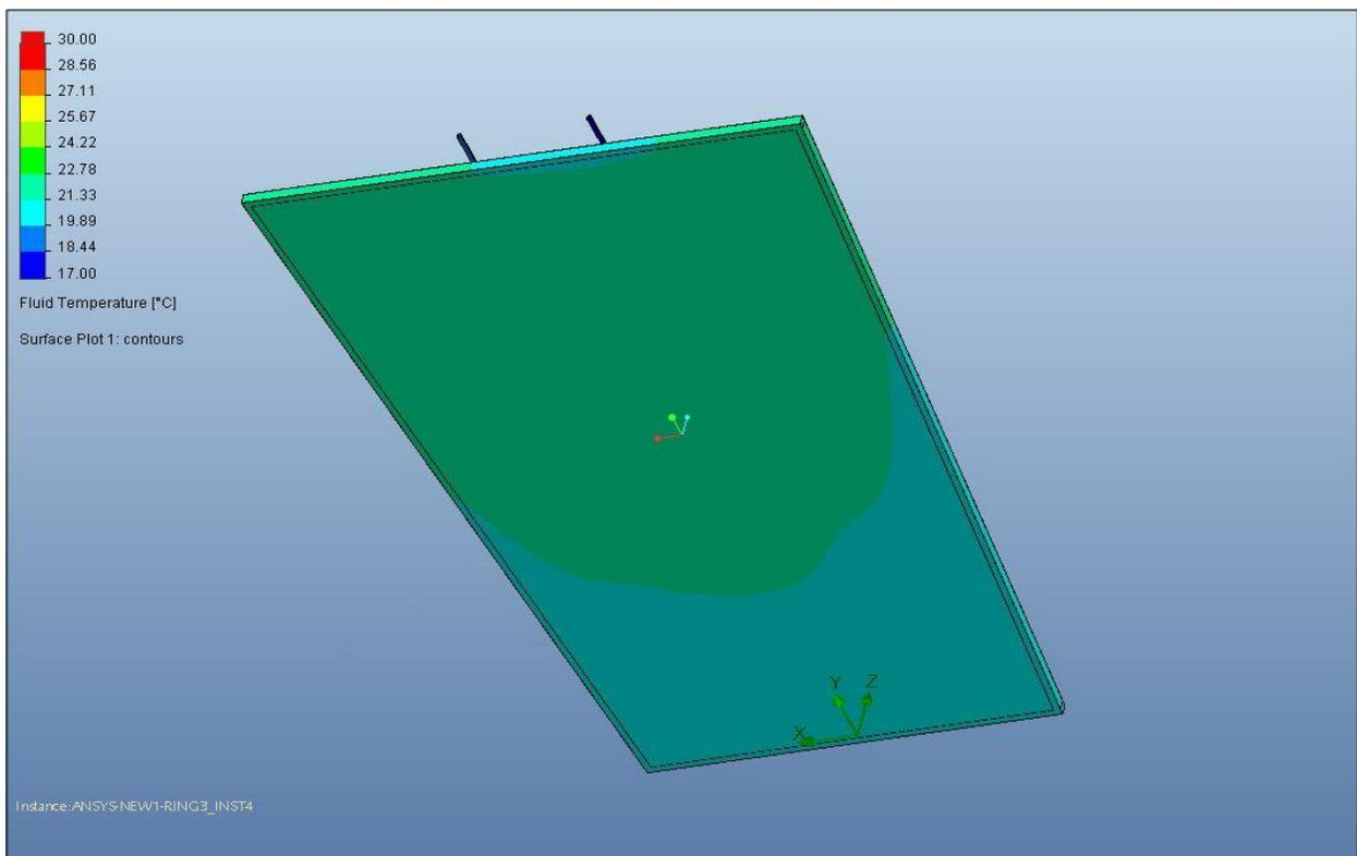
Figure 9 Temperature distribution on the top side of the bottom honeycomb panel (simulation).
