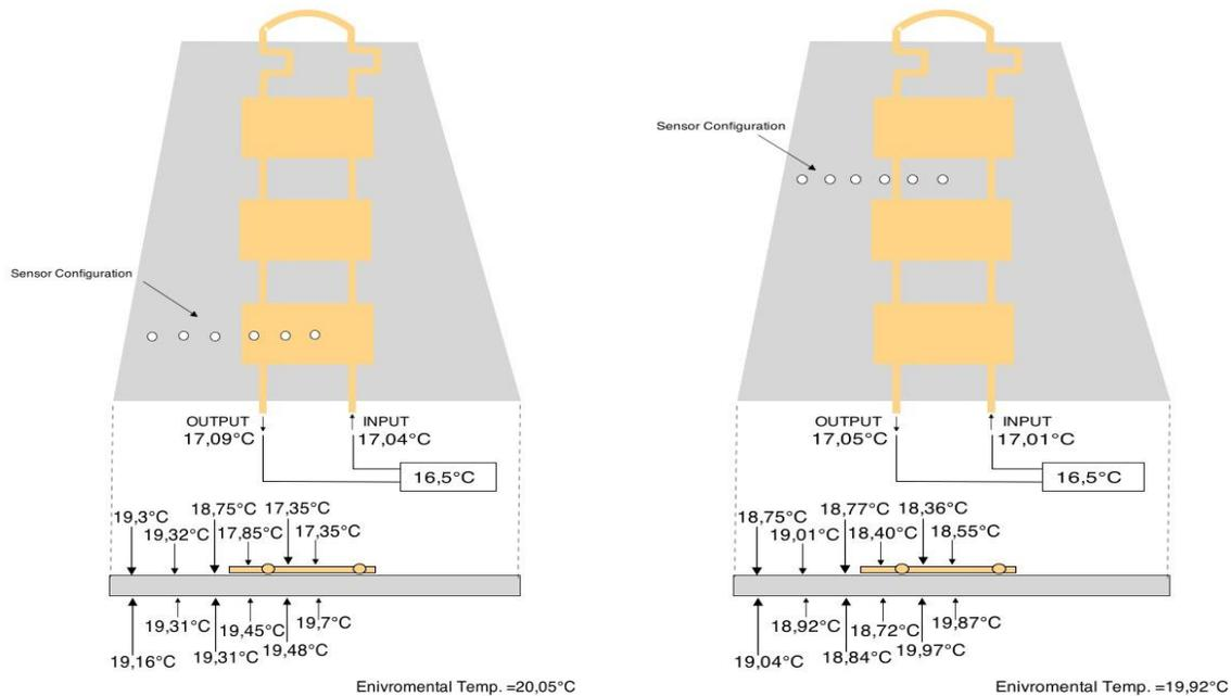
Figure 11 Temperature of the outer surfaces of the honeycomb in two different regions of the RPC.
