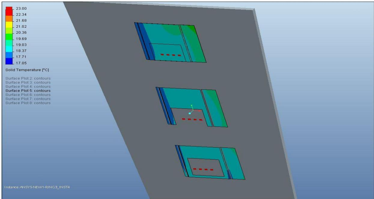
6 Temperature distribution on the copper plates (simulation).
