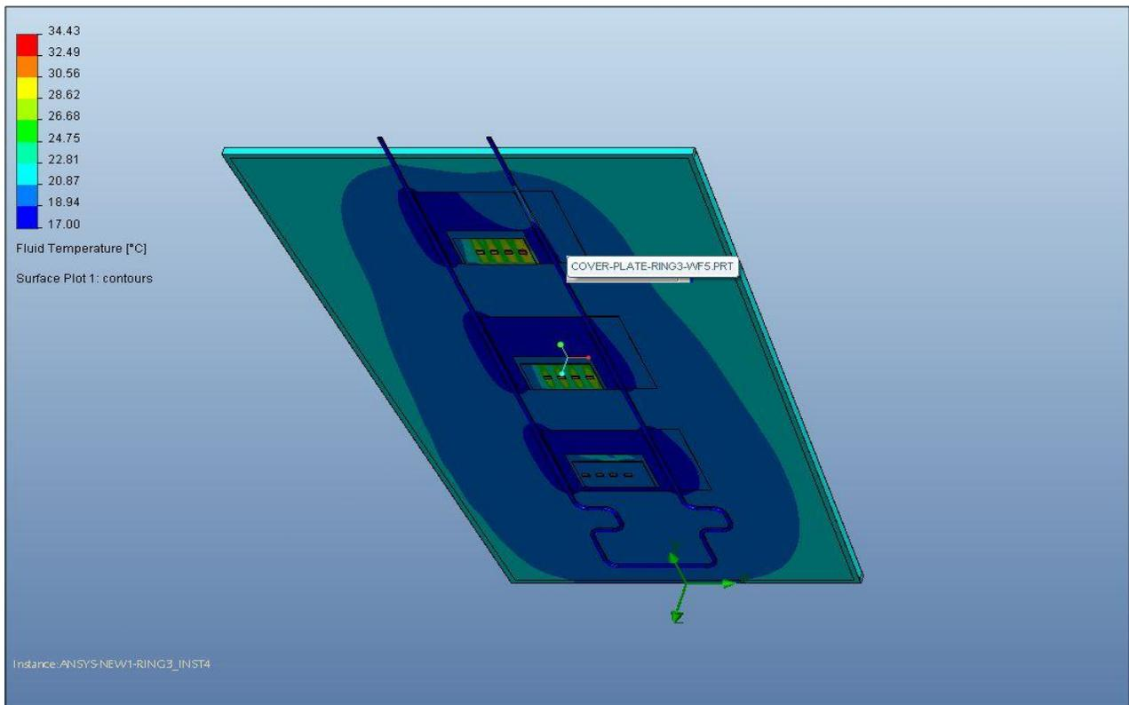
Figure 7 Temperature distribution of the top side of the honeycomb panel (simulation).
