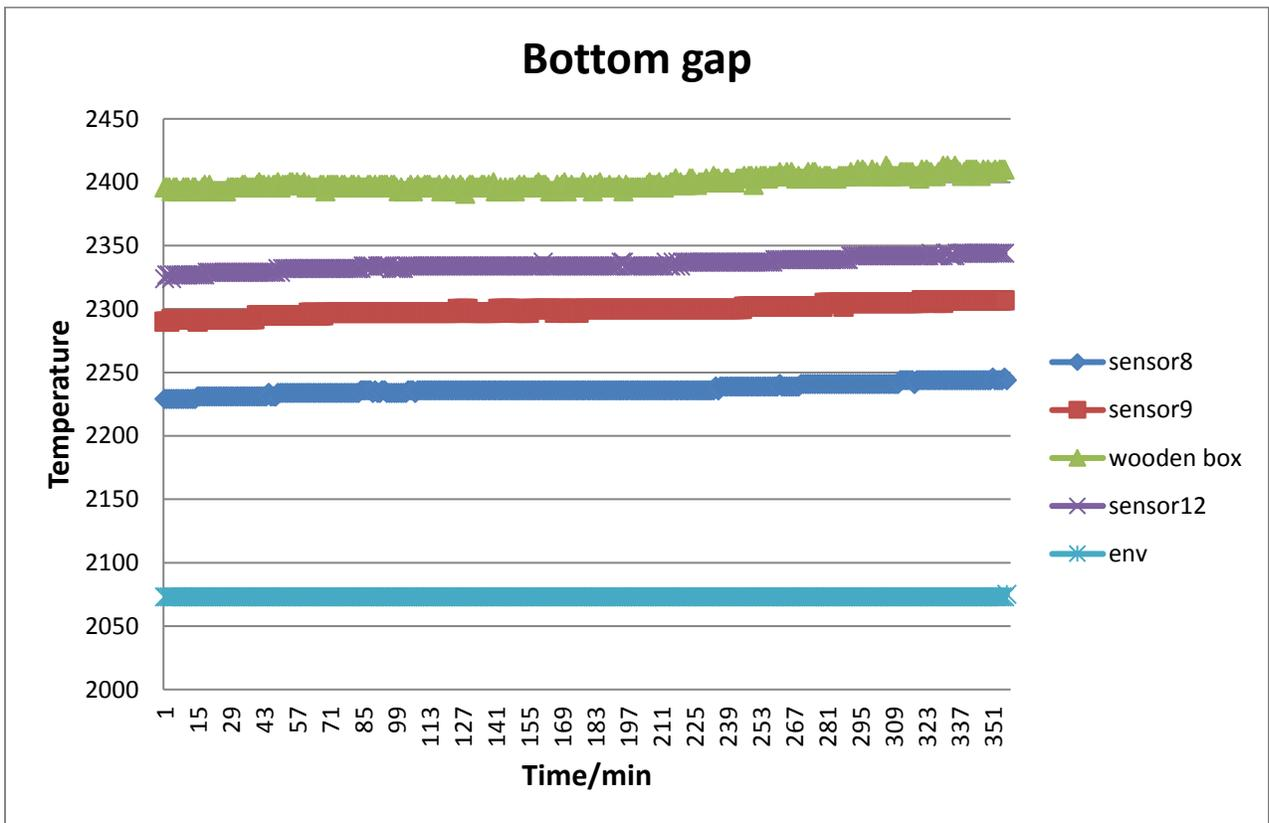
Figure 15 Temperature of the sensors for cooling at 18°C and flow rate 2l/min
