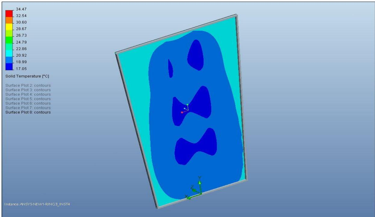
Figure 8 Temperature distribution on the bottom side of the top honeycomb panel (simulation)
