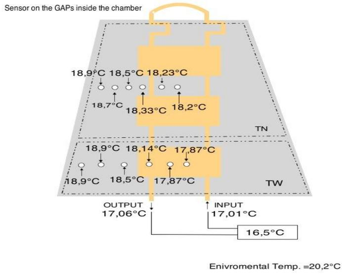
Figure 12 Temperature of the top surface of the top Baklite gap.
