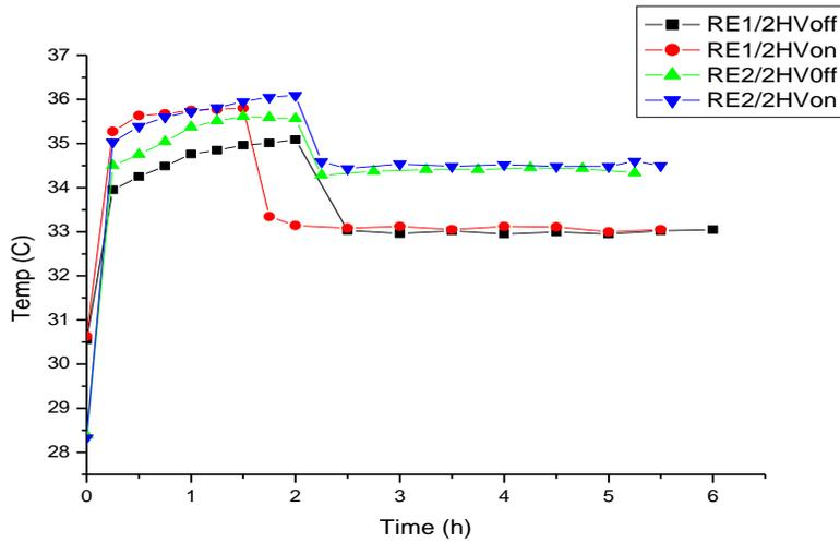
Figure 3. The variation of the FEB temperature with time for both RE1/2 and RE2/2 with HV on and off and cooling (16 °C) off at the first part of the graph and on at the second part.
