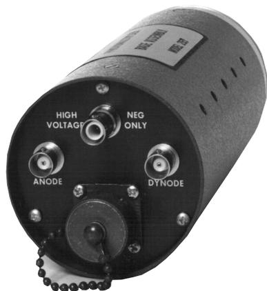
The ORTEC Model 269 Photomultiplier Base structure is a mechanical assembly and resistive voltage divider network, with appropriate capacitive-decoupling for operation of 14- and 12-stage PMTs that fit standard 20-pin sockets, including:
