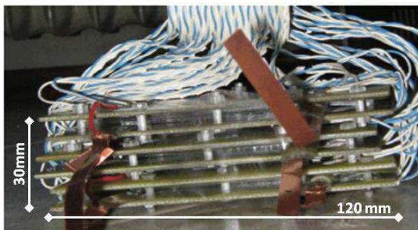
**Figure 8.** The MGIC RPCPET prototype (small).
