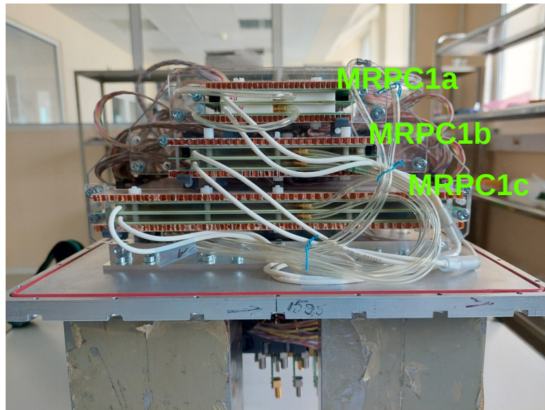
Direct flow MSMGRPC stack
