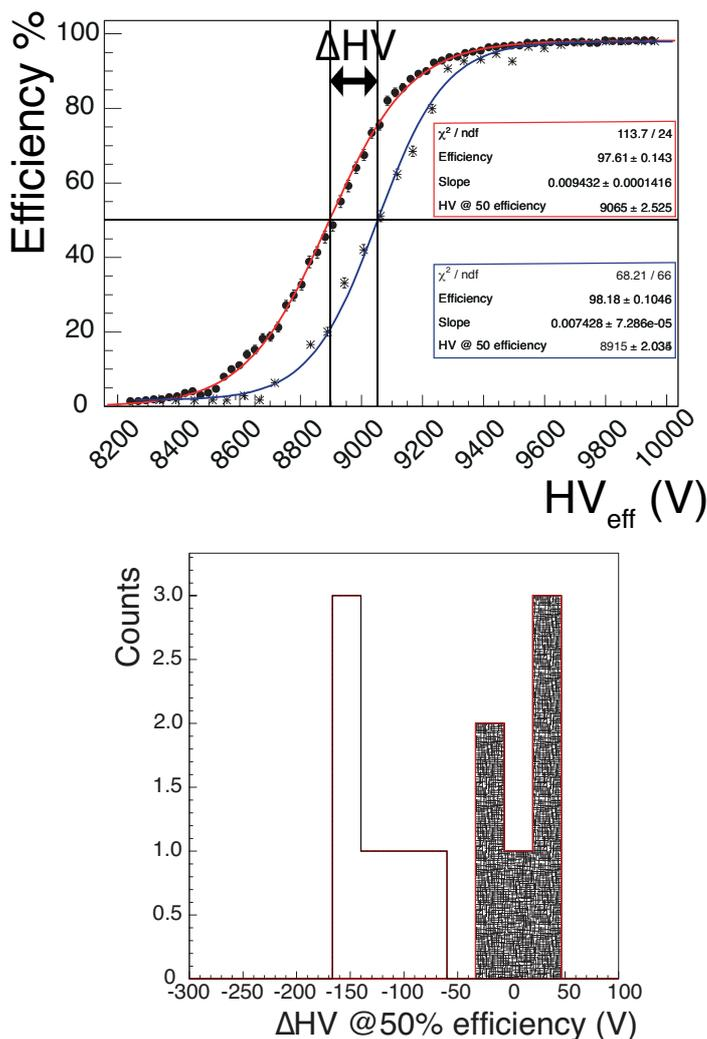
**Figure 4.** (top) Typical GGM high voltage scan performed during January 2010 (star) and April 2011 (full circle). (bottom) Difference in voltage between the HV scans performed in April 29th 2011 (correct gas mixture) with respect to and March 3th 2011 (empty histogram - wrong gas mixture) and January 10th 2010 (hatched histogram - correct gas mixture).
