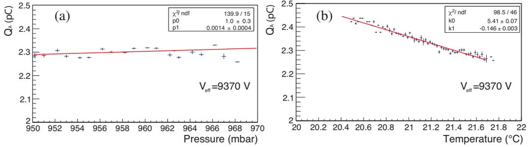
**Figure 2.** (a) Correlation plot between GGM RPC anodic charge against environmental pressure. (b) Correlation plot between GGM RPC anodic charge against environmental temperature. The meaning of fit parameters  $p_0, p_1, k_0, k_1$  is described in the text.
