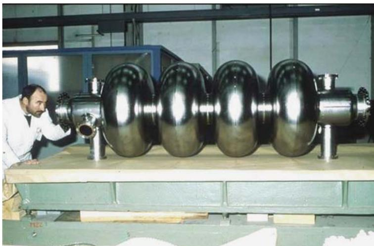
**Fig. 6.9** A superconducting cavity with four niobium accelerating cells
