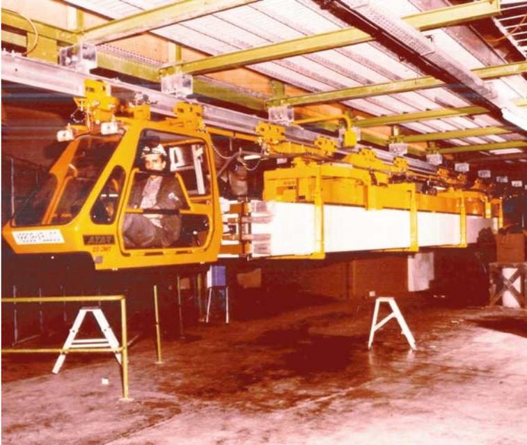
**Fig. 6.11** Monorail train for the transport of bending dipole magnets
