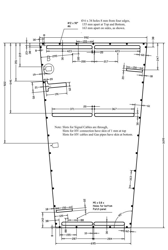
Note: Drawing is such that we are looking at the top pannel from outside the chamber
