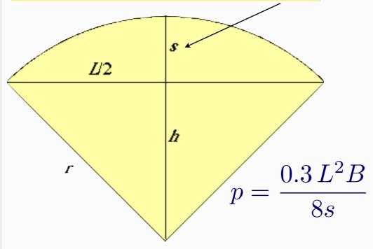
$$\frac{\delta p}{p} = \underbrace{\frac{8}{0.3} \underbrace{\frac{1}{L^2 B}} p \, \delta s}_{p \, \delta s} = \underbrace{\frac{\delta s}{s}}_{s}$$
