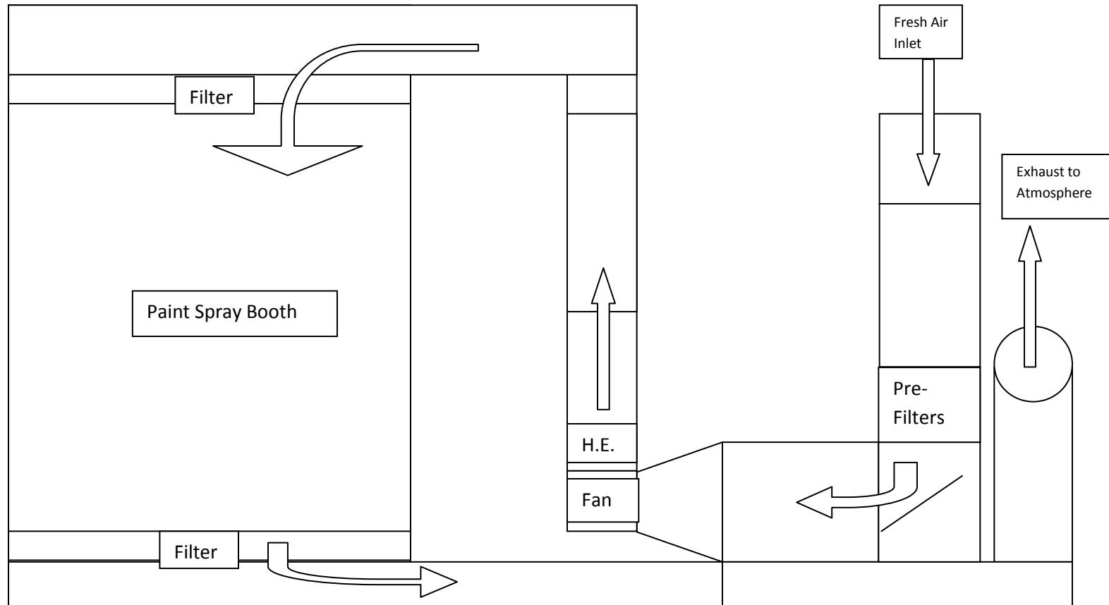
Recirculating of warm air/ Recirculation d'air rechauffer
