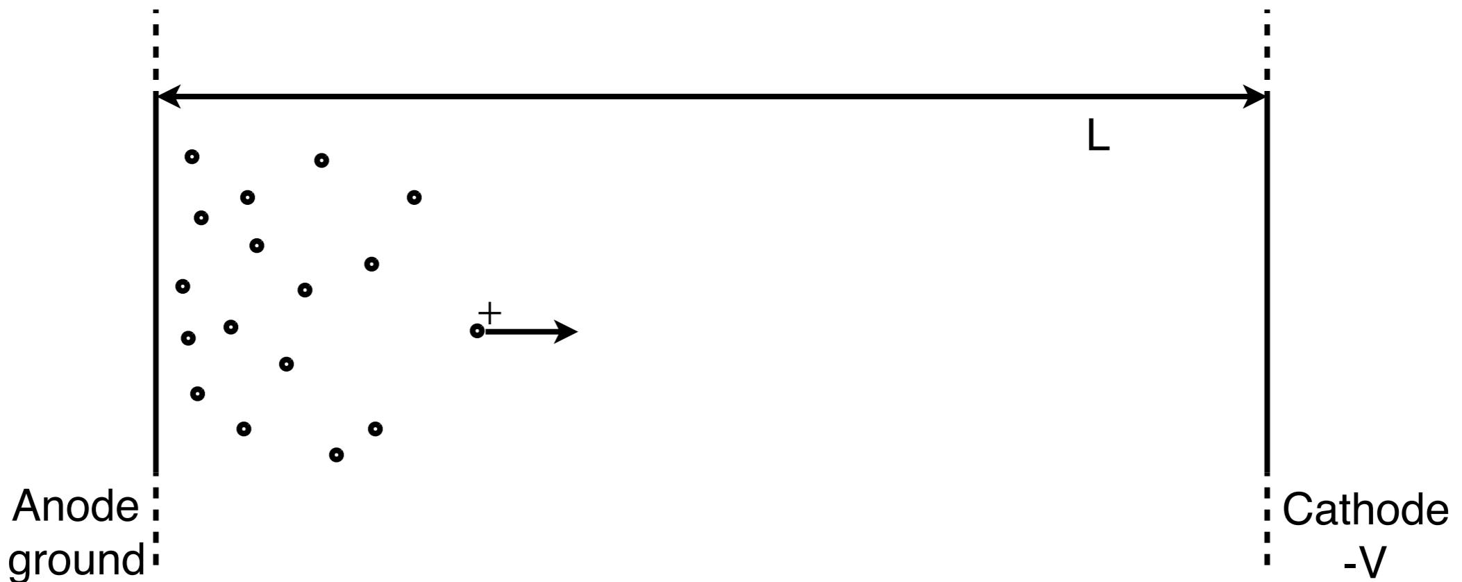
Infinite parallel plates at distance  $L$  with a potential difference of  $\Delta V$
