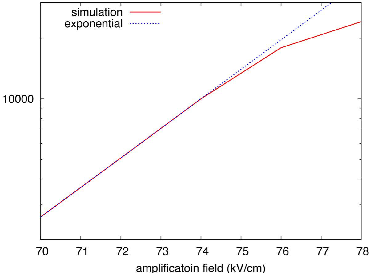
Ions moving towards the entrance of the hole reduce the amplification field affecting the multiplication of the forthcoming electrons
