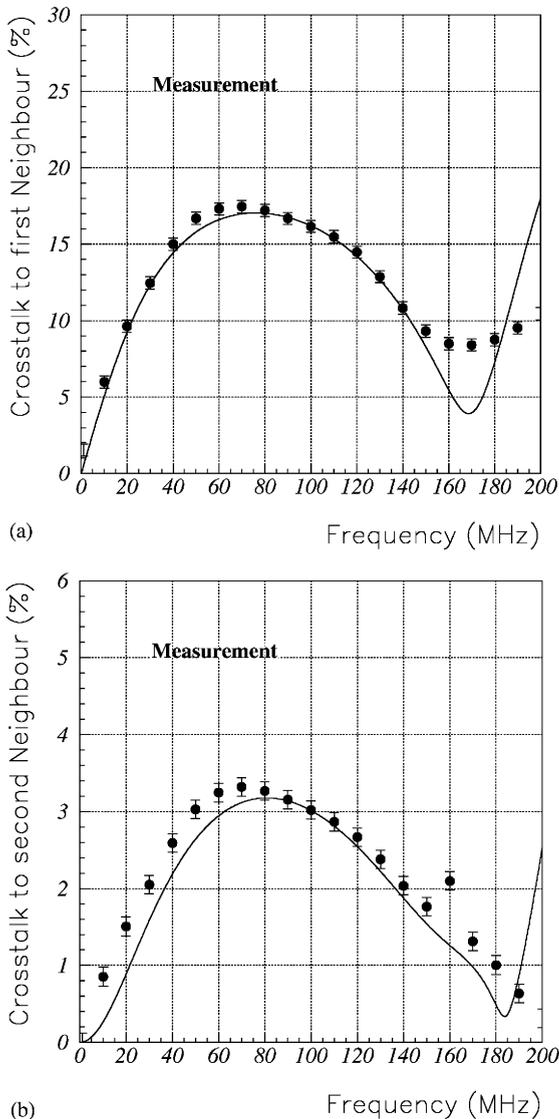
Fig. 16. Measurement of the crosstalk for an RPC with the geometry similar to Fig. 9. A voltage sine wave was put on one strip and the amplitude on the first (a) and second (b) neighbour strip was measured. The Bakelite was assumed to have  $\epsilon = 10$ , losses were neglected. The solid line shows the simulation, the points show the measurement. For frequencies  $< 200$  MHz the agreement is acceptable.
