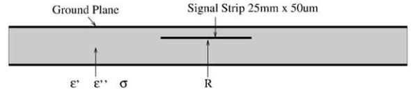
Fig. 14. Homogeneous transmission line with a single lossy conductor and a lossy surrounding medium.
