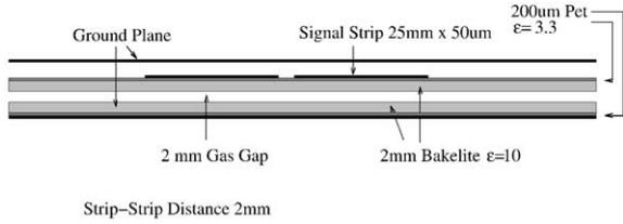
Fig. 6. RPC with two strips. The dielectric properties are *not* uniform in the area where the waves propagate which leads to different propagation velocities.
