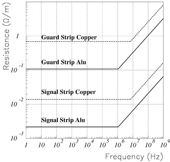
Fig. 15. Conductor resistance assuming all the current to flow within one skin-depth for the RPC geometry in Fig. 9.
