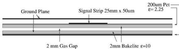
Fig. 2. Cross-section through a RPC with a single signal strip. The current signal is induced by the avalanche electrons moving in the gas gap.
