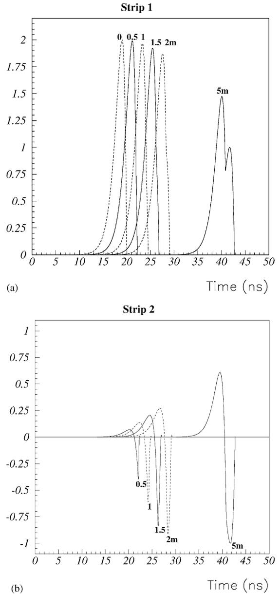
Fig. 7. Current pulses running along the two strips of the RPC shown in Fig. 6. The labels show the distance of the induced signal from the amplifier side. (a) Signal on the strip where the current is induced. One can see that the two ‘modes’ are dispersing after some distance. (b) Signal travelling on the neighbouring strip. At the position where the signal is induced the crosstalk signal is zero, as the modes are dispersing the crosstalk increases.
