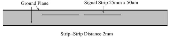
Fig. 3. Cross-section through a homogeneous transmission line with two strips.
