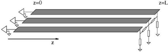
Fig. 1. Two-dimensional multi-conductor transmission line. The formalism for 2-dimensional transmission lines applies if the cross-section is independent of  $z$ . The cross-section of the individual conductors can be different.
