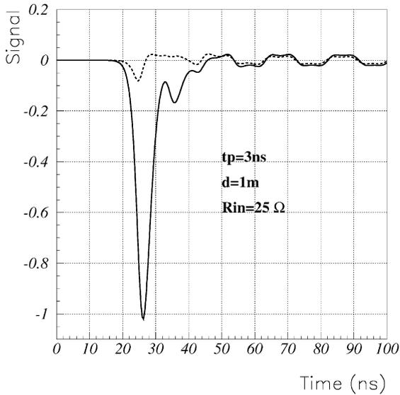
Fig. 11. Signal (solid line) and crosstalk (dashed line) for the scenario where the RPC strips are terminated at  $25\Omega$  and the intermediate strips are grounded on both sides. As expected we find reflections.
