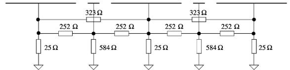
Fig. 10. Ideal termination for the RPC with many strips calculated from Eq. (9). All other interconnections are  $> 25\text{k}\Omega$  and have negligible effect.
