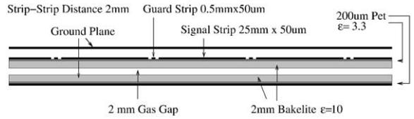
Fig. 9. RPC geometry with many strips and a guard strip to reduce the strip–strip coupling.
