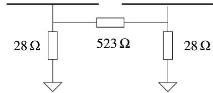
Fig. 4. Termination network for a double strip RPC calculated from Eq. (9). In order to perfectly terminate a multi-conductor transmission line one has to interconnect all the lines.
