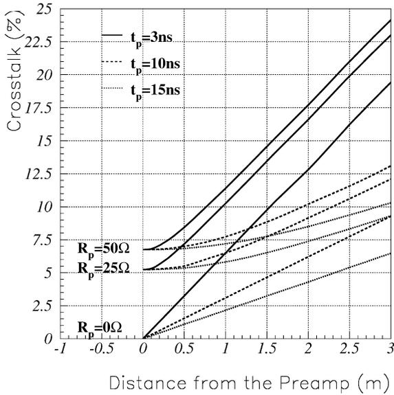
Fig. 8. Crosstalk for different preamplifier input resistances and peaking times as a function of distance from the amplifier side (RPC shown in Fig. 6). For small distances the pulses do not disperse and the crosstalk is given by Eq. (15), independent of the amplifier speed. For fast amplifiers the crosstalk increases strongly with the distance. In the limit of very long peaking times the crosstalk would become independent of the position.
