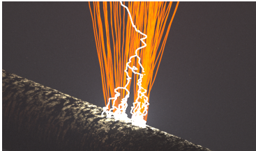
Figure: Simulation of avalanche in proportional counter.
