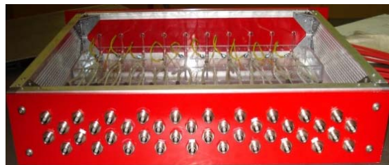
Figure 4.1: HV distribution box
