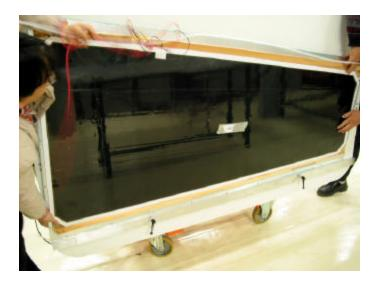
Adjust the height of the RT to some few mm higher than the marble .Slide the HCP and gap onto the assembly table. The HV connexion is no longer apparent!
