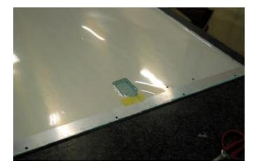
The PET/Cu combined sheet must be creased along its long sides as shown.
