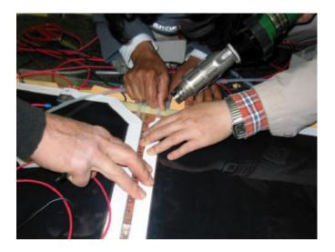
Secure the two longest gas pipes in place using tape, to ensure that they are not tapped during the top HCP mounting. Perform a visual inspection of all pipe connections to be sure non have been left out and that each gap layer has its own circuit.
