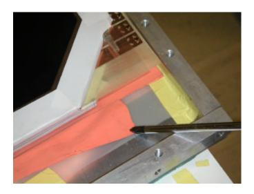
Cut out the Copper and top PET film around the inter gap gas connexions. Leave the bottom intact as shown.
