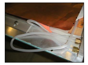
Cut to length the inter gap gas links and push onto their gas gap connexions by pre heating the PE pipe using the hot air gun adjusted to #5, not hotter, patience.
