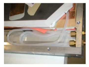
Be sure that the pipes are not twisted as shown below !
