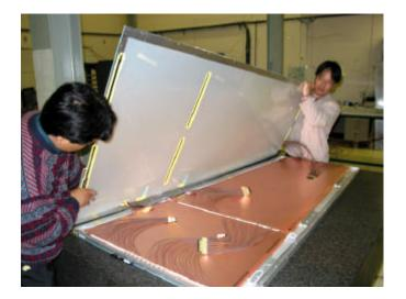
Continue to descend the panel passing each AB through their slots as they come within reach. Do not allow the cables to snag during this operation. Take care not to twist and pull on them as the y pass through the slots.
